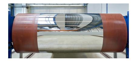
"The endless nano-polished belt is characterized by its high-quality belt characteristics and its long lifetime. A specially developed surface protection leaves no residue on the steel belt surface and, coupled with nano-technology, allows an immediate use of the belt. This "ready-to-use model" is unique in the world and demonstrates our innovative edge."
