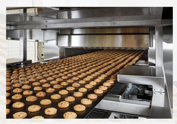
© Haas Meincke's state of the art test bakery in Skovlunde, Denmark. The test oven is equipped with a solid CARBO 13 steel belt from Berndorf Band.
