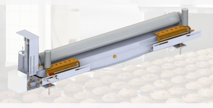
"The *berntrack*® system can significantly reduce downtime and increases the production quality, especially in machines which do not have an active belt tracking system. *berntrack*® detects even the slightest deviations in the belt run due to mechanical or thermal conditions and compensates them immediately."
